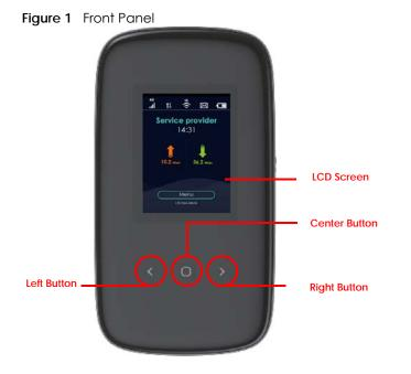
You can use the center, right, and left buttons to navigate the LCD screen.
