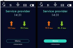
• The Menu screen appears. Press the left or right button to scroll up and down and then press the center button to select an option.
