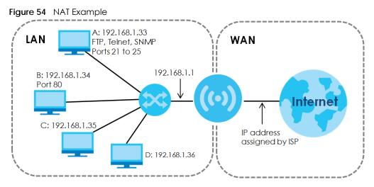
Note: You must create a firewall rule in addition to setting up NAT, to allow traffic from the WAN to be forwarded through the LTE2566-M634.
